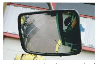
Wide angle mirrors aren't limited to use on trucks only, they are used in different applications to improve safety. The class IV & V approved M430CE can be seen above mounted onto a piece construction equipment. It is being used to help meet a visibility standard.
