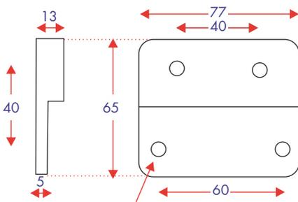
4 x 7 DIA HOLES SPACED AS SHOWN
