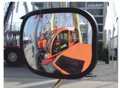
Safety mirrors are now widely used on all different types of machine and application. At one time any mirror would do but these days a more considered approach is taken. Stricter visibility standards, designed to reduce and prevent accidents, mean better quality solutions are now required. Ashtree products are specially designed to meet these stricter requirements.
