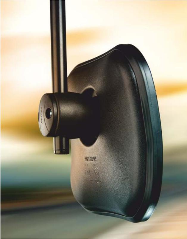
There are 3 classes of wide angle mirror and they each fulfil a different role. The newest, class VI, mounts over the drivers screen so the front of the truck can be seen. All the children in the photo below were completely invisible to the driver without a Class VI mirror.
