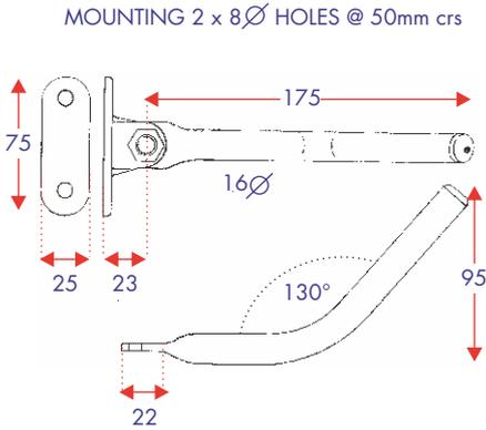
MOUNTING 2 x 8Ø HOLES @ 50mm crs
