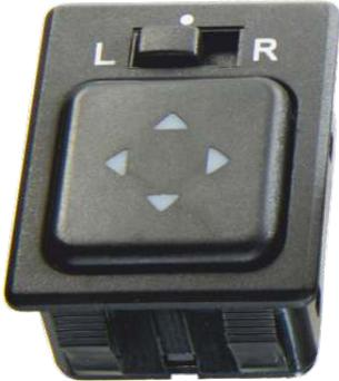
4 way mirror adjustment switch (both sides). Complete with 2 metres of cable. Dimensions: 47mm x 38mm to fit hole 44mm x 33mm
