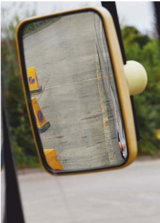
The image to the left shows the drivers view using one of the most popular mirrors on UK buses. The road cones show the outer limits of the drivers visibility. Some other mirrors used are even smaller than this, further restricting visibility.
