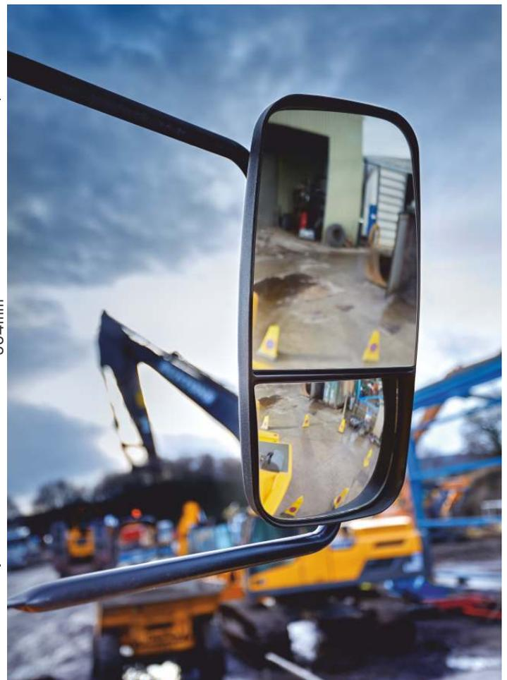
This image shows the extra visibility we got when the M926CE/M925CEH was mounted onto a wheeled loader. Visibility right up to the rear axle was possible, this is the area that most standard mirrors do not pick up.
